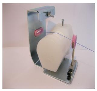
This yarn lubrication device can be applied both on knitting machines than on circular knitting machines. The yarn during the phase of "knitting" flows on a specific porous ceramic sintered material which allows a perfect yarn lubrication increasing its smoothness and reducing broken needles and machine downtime, lubricating itself perfectly and dramatically decreasing the coefficient of friction of the yarn, increasing its smoothness.
