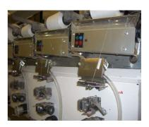
LUBRIFIL can be used on all types of yarn without any limits in material and colour. The installation on the machine is simple, fast and thanks to the experience of tens of thousands of winding units already in operation, the NUOVA RIMATES provides a kit of brackets ready for use.
