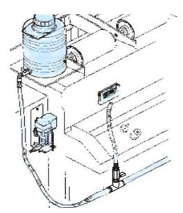
The lubrication of the yarn is obtained by exploiting the movement of yarn traverse during the winding operation. The yarn is in contact with a special material which could be in nylon, polyester, stainless steel, or porous sintered ceramic.
